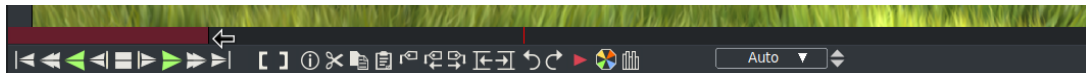
Figure 2.19: A left-facing arrow on the right side of the reddish slider bar is used to drag the bar.
