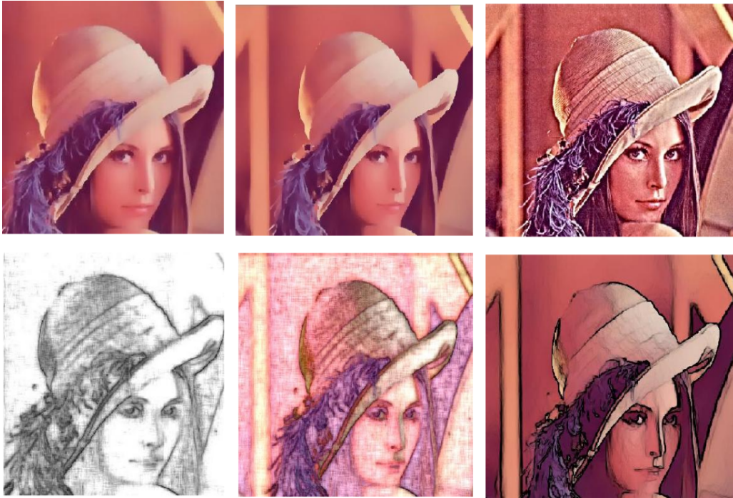
Figure 9.83: Clockwise: Edge Smooth and Recursive ; Detail Enhance ; Stylization ; Color and Pencil Sketch
